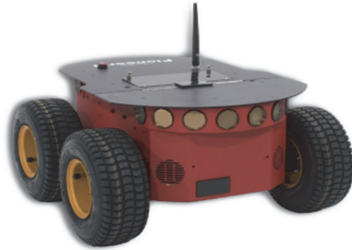
1. ábra PIONEER 3-AT mobil robot
