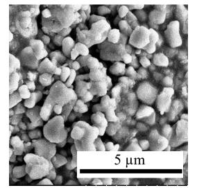
SrTiO<sub>3</sub> after Phenol degradation
