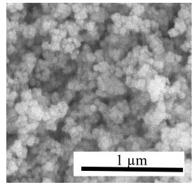
The SEM micrograph of synthesized reference SrTiO<sub>3</sub> showed that there significant were no changes in morphology after degradation.
