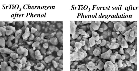
The SEM measurements of the reference SrTiO<sub>3</sub> showed that the particles underwent a slight aggregation after phenol degradation. Forest soil extract disaggregated the particles into smaller chunks, but there were no significant changes in the morphology.
